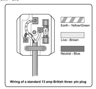
The wire coloured green and yellow must be connected to terminal marked with the letter E, coloured green and yellow or marked with the earth symbol:
